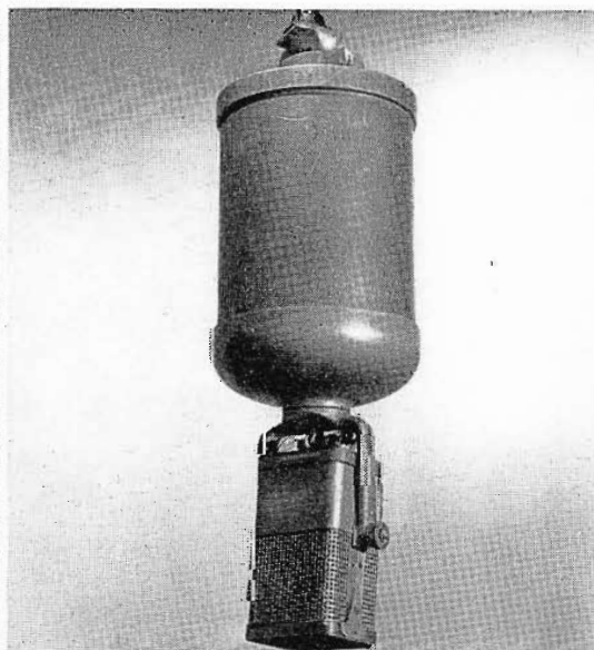
1930 An early model Ribbon Microphone (Velocity type). Note attached pre-amplifier and use of electromagnetic field.
