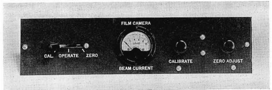
FIG. 13. Beam Current Metering Control Panel.
